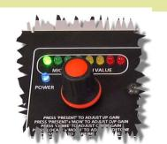
Microphone Level Meter An eight LED front panel multipurpose indicator is used to indicate the outgoing microphone level.
